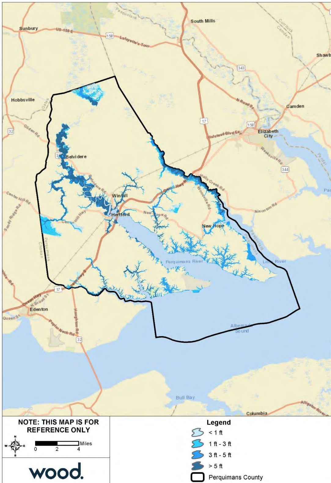
Figure 4.36 – Flood Depth, 100-Year Floodplain, Perquimans County
